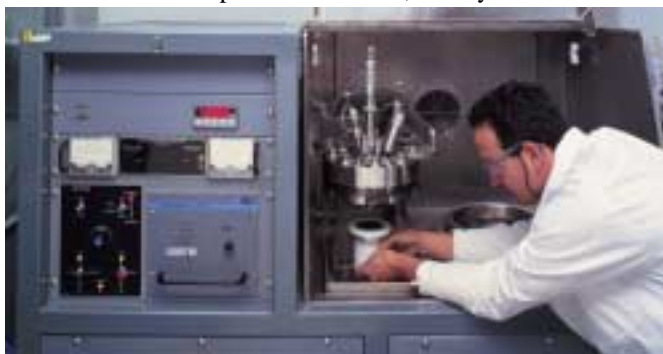
The Centre's Dr Ulf Kreher carrying out experimental work on the Microwave Batch Reactor.
